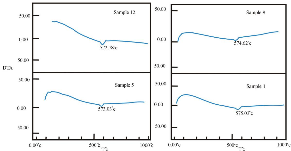
Figure 2. Differential thermal analyses (DTA) curves showing the thermal behavior of  $\alpha$ -quartz samples and change of  $\alpha$ -quartz to  $\beta$ -quartz at Marwat Alimikan area
