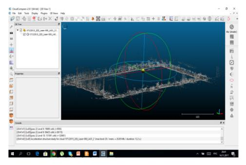
Figure 7 – Program for compare the obtained digital models of Cloud Compare
