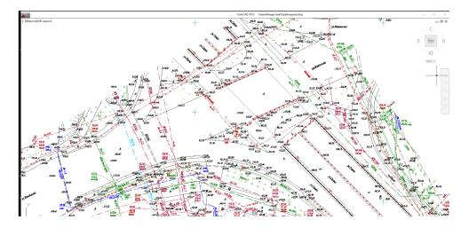
Figure 2 – Fragment of tacheometric survey of the road section of Almaty city
